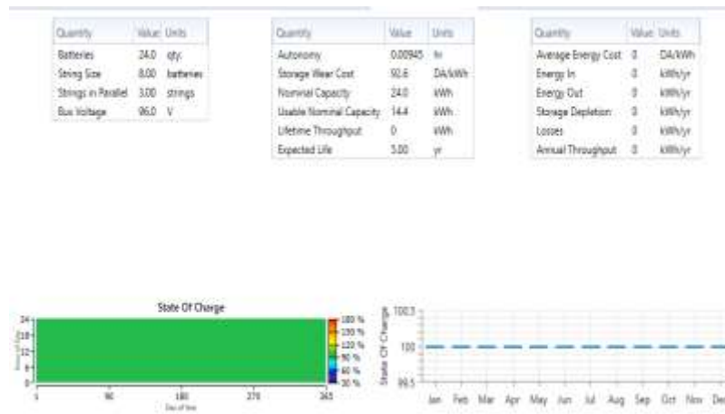
Figure 10. Average daily and monthly state of charge of the battery bank
